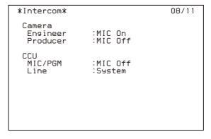
Camera Engineer: Camera microphone status of the ENG line of the camera
