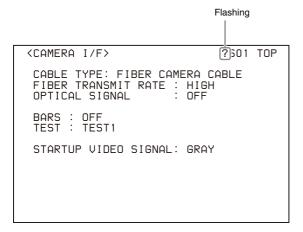
**2** Turn the CONTROL knob to change the displayed page to the desired page, then press the CONTROL knob.
