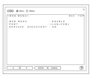
Click the  $\triangle$  (up) button and  $\nabla$  (down) button at the bottom of the screen to switch between screens. Clicking the ENTER button applies/executes a setting. Clicking the CANCEL button cancels a setting.
