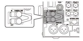
The CAMERA SMF IN connector inputs the video signal from the camera, audio (microphone) signal, HD-TRUNK signal, and NETWORK TRUNK signal.
