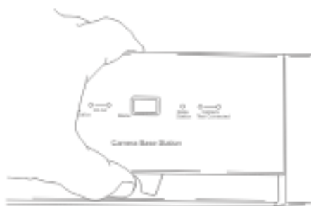
Figure 6-2. Removing the Power Unit
